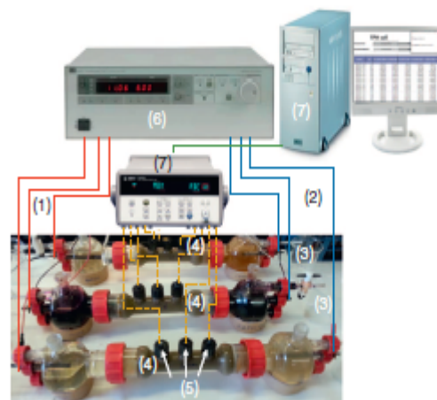
Fig. 1. Experimental set-up for the simulated bench scale in-situ experiments: (1) anode, (2) cathode, (3) electro-osmotic flow reservoir, (4) soil sample, (5) auxiliary electrodes, (6) power supply, (7) data acquisition system.
